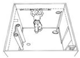
Make a guide mark on what will be the uppermost edge of wall covering (corresponding to the midpoint of the roll length or at the suitable starting place, as appropriate).
