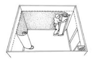
Starting from the centre of the cut length, work upwards and downwards. Make sure that the tool you choose for smoothing out the wall covering does not damage it. Heat should not be used when working with the wall covering except for external corners.
